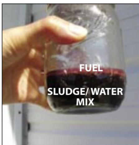
THIS SAMPLE CONTAINS HEAVY AMOUNTS OF DEGRADED FUEL PRODUCTS AND WATER.
