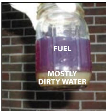
BY THE SAMPLE TO LEFT, THIS TANK HAS A PROBLEM WITH EXCESSIVE WATER ACCUMULATION. YOU CAN ALSO DETECT THIS MUCH WATER WITH WATER-INDICATING PASTE ON A STICK.
